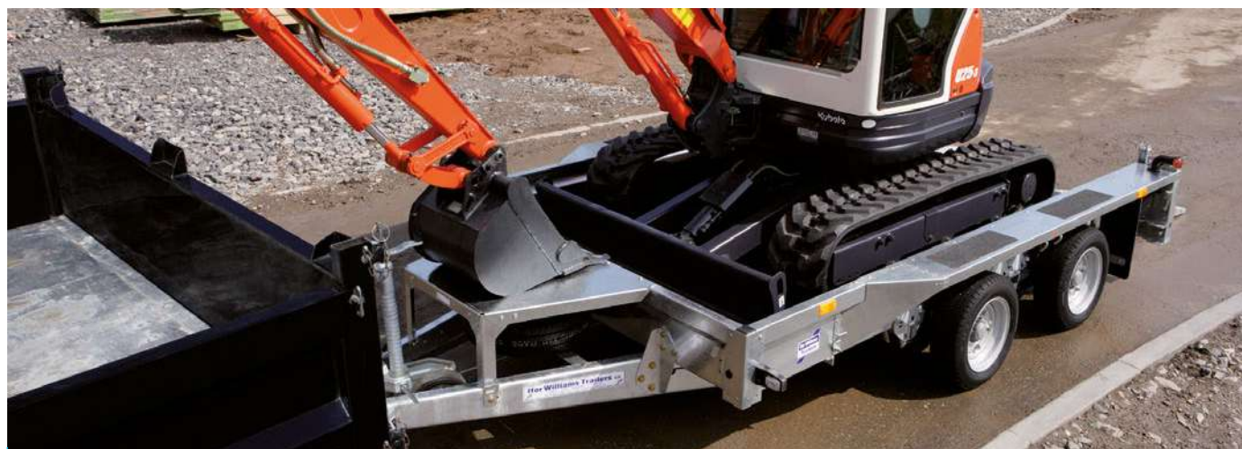
GX106 with skids and integrated rear supports
